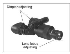
To focus the NVG-7, first you will need to adjust the diopter. Simply turn the diopter clockwise until it stops. Then, while looking throught the diopter at an object, slowly turn the diopter back counter clockwise until the grain in the image is sharp.
